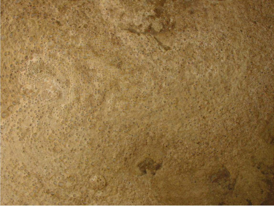
Photo taken within 5 minutes of adding Noflex Digestor The sludge immediately started foaming after the Noflex was added. Note: This continued to look like this for the next 4 hours while I was at the site.
